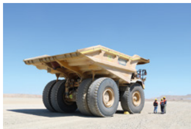
Aktogay 793D haul truck with lightweight tray, 236 t payload
